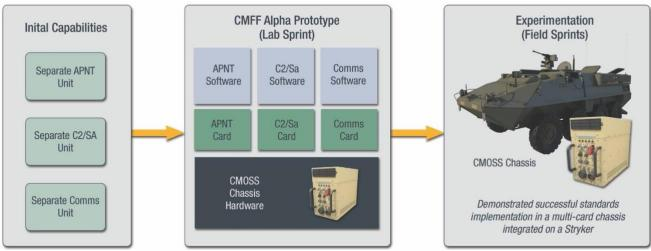
Figure 5: CMOSS Architecture
